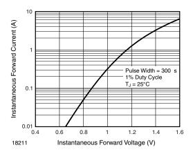
Fig. 2 - Typical Instantaneous Forward Characteristics for GLL4763
