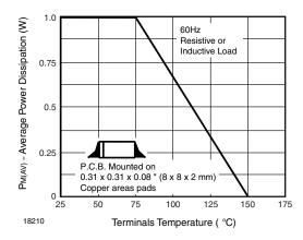
Fig. 1 - Maximum Continuous Power Dissipation
