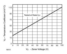
Fig. 3 - Typical Temperature Coefficients
