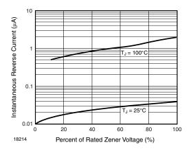
Fig. 5 - Typical Reverse Characteristics
