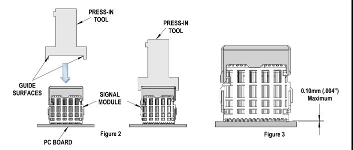
3. Using the application tool and an appropriate press, seat the Signal module until there is less than 0.10mm (.004 in.) clearance between the bottom of the plastic housing and the surface of the PCB. See Figure 3.
