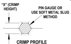
Use gauge pins or soft metal slug (solder) method to measure the "X" dimension. Verify the tooling crimp height calibration by referring to the Go/No Go dimensions shown in the chart below.
