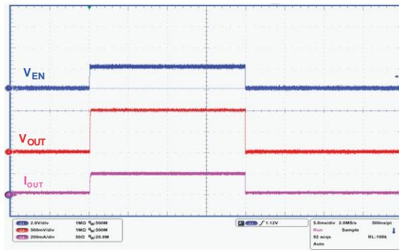
$V_{IN}=2V$ ,  $V_{EN}=0V$  to  $V_{IN}$ ,  $I_{OUT}=0.2A$ ,  $V_{OUT}=1V$ ,  $T_r=5\mu s$
