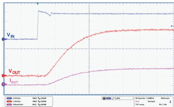
$V_{IN} = V_{EN}$  from 0V to 5.5V,  $I_{OUT} = 0.2A$ ,  $V_{OUT} = 5V$ ,  $T_r = T_f = 5\mu s$
