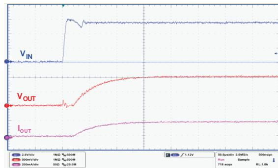
$V_{IN} = V_{EN}$  from 0V to 5.5V,  $I_{OUT} = 0.2A$ ,  $V_{OUT} = 1V$ ,  $T_r = T_f = 5\mu s$
