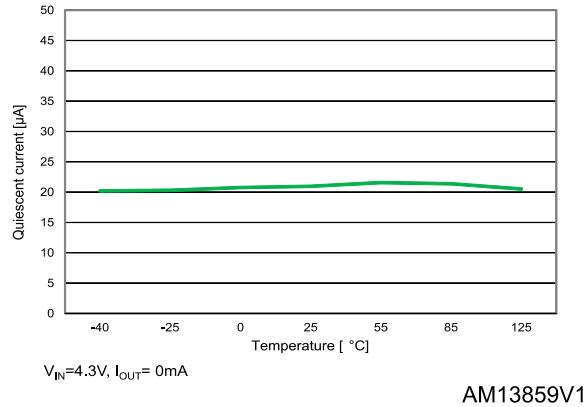
**Figure 9: Quiescent current vs. temperature ( $I_{OUT} = 200 \text{ mA}$ )**
