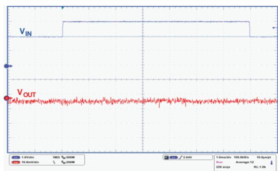
$V_{IN} = V_{EN}$  from 2V to 3V,  $I_{OUT} = 10mA$ ,  $V_{OUT} = 1V$ ,  $T_r = T_f = 5\mu s$
