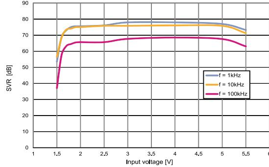
$I_{OUT}=30mA$ ,  $V_{OUT}=1V$ ,  $C_{OUT}=1\mu F$
