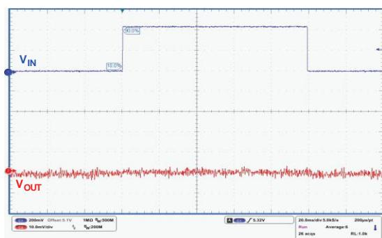
$V_{IN} = V_{EN}$  from 5.1V to 5.5V,  $I_{OUT} = 10mA$ ,  $V_{OUT} = 5V$ ,  $T_r = T_f = 5\mu s$
