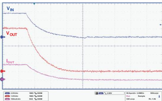
$V_{IN} = V_{EN}$  from 5.5V to 0V,  $I_{OUT} = 0.2A$ ,  $V_{OUT} = 5V$ ,  $T_r = T_f = 5\mu s$
