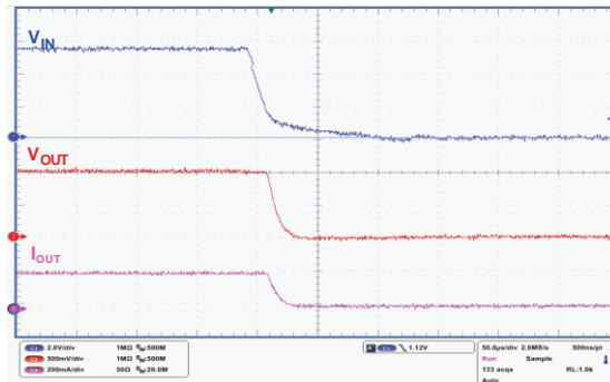
$V_{IN} = V_{EN}$  from 5.5V to 0V,  $I_{OUT} = 0.2A$ ,  $V_{OUT} = 1V$ ,  $T_r = T_f = 5\mu s$
