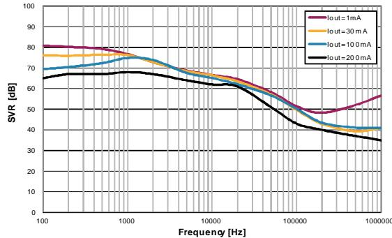
$V_{IN}=2V \pm 20mV$ ,  $V_{OUT}=1V$ ,  $C_{OUT}=1\mu F$
