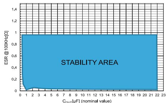
$V_{IN}$  from 2 to 5.5V,  $I_{OUT}$  from 0 to 200mA,  $C_{IN}=1\mu F$
