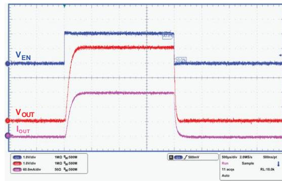
$V_{IN}=5.5V$ ,  $V_{EN}=0V$  to  $2V$ ,  $I_{OUT}=0.2A$ ,  $V_{OUT}=5V$ ,  $T_r=5\mu s$
