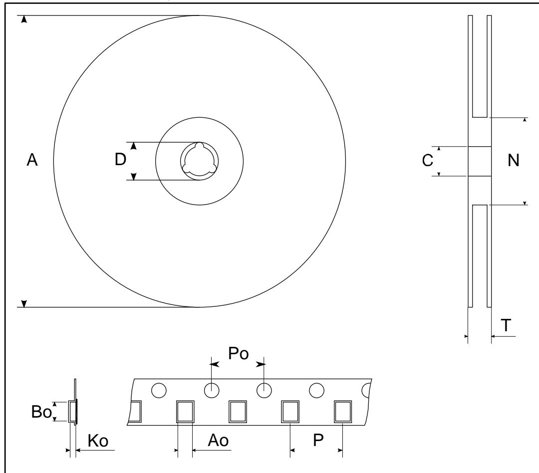
Table 9: SOT23-5L tape and reel mechanical data
