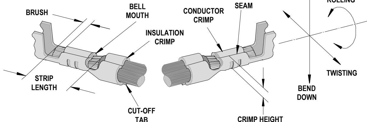
The above terminal drawing is a generic terminal representation. It is not an image of a terminal listed in the scope.
