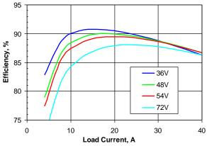
Figure 3. Efficiency vs. load current and ambient temperature for SQE48T40015 converter mounted vertically with Vin=48V and air flowing from pin 3 to pin 1 at 200LFM (1.0m/s).
