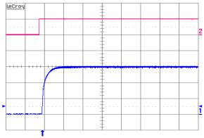
Figure 7. Turn-on transient at full rated load current (resistive) plus 10,000  $\mu$ F at Vin = 48 V, triggered via ON/OFF pin. Top trace: ON/OFF signal (5 V/div.). Bottom trace: Output voltage (0.5 V/div.). Time scale: 5 ms/div.
