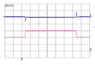
Figure 8. Output voltage response to load current step-change (20 A – 30 A – 20 A) at Vin = 48 V. Top trace: output voltage (100 mV/div.). Bottom trace: load current (10 A/div.). Current slew rate: 0.1 A/ $\mu$ s. Co = 1  $\mu$ F ceramic. Time scale: 0.2ms/div.
