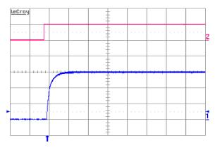
Figure 9. Output voltage response to load current step-change (20 A – 30 A –20A) at Vin = 48 V. Top trace: output voltage (200 mV/div.). Bottom trace: load current (10 A/div.). Current slew rate: 2.5 A/ $\mu$ s. Co = 470  $\mu$ F POS + 1  $\mu$ F ceramic. Time scale: 0.2 ms/div.
