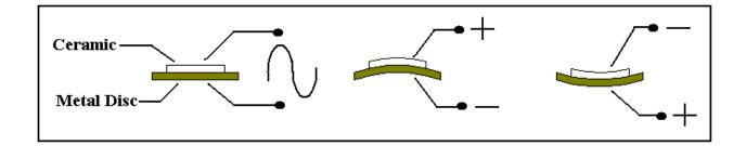
The above picture shows a bare piezoelectric sounder element. By applying a sinusoidal waveform at an appropriate frequency, the transducer will physically deflect in one direction and then in the opposite direction following the shape of the input wave-form. If this oscillation occurs in the audible frequency range (1 Hz to 20 kHz), then air pressure waves are produced that the human ear interprets as an audible sound.
