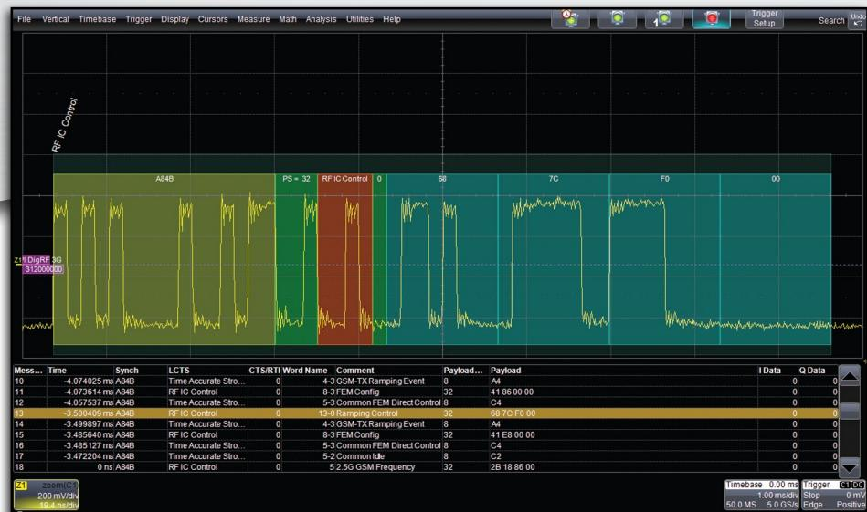
View an entire DigRF 3G burst using intuitive decoding and table display. Click the table to view a zoom of a particular packet.
