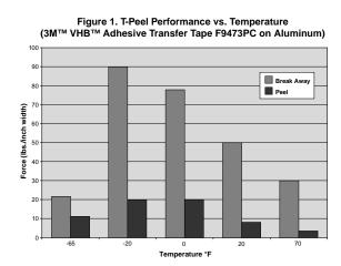
when high impact stresses along with high frequencies are encountered. At low temperatures, the tape becomes very firm and glassy; the ability to absorb impact energy is reduced.
