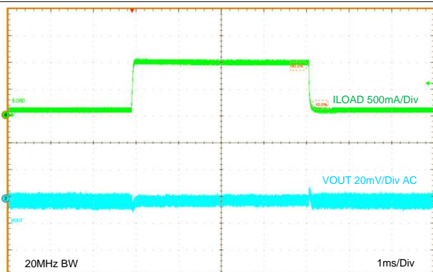
Figure 60. Load Transient V_{OUT} = 3.3\text{ V}
