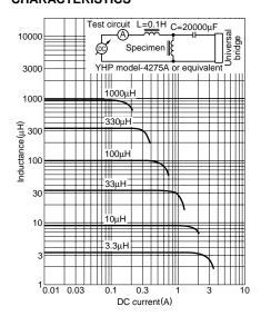
Test equipment L:YHP 4194A IMPEDANCE GAIN/PHASE ANALYZER or equivalent (Measured at 1kHz/0.5V)
