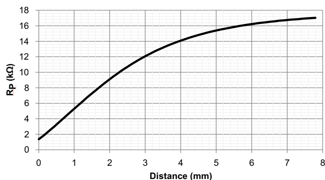
Figure 52. Example R_P vs. Distance with a 14-mm PCB Coil and 2mm Thick Stainless Steel Target
