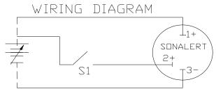
IF S1 IS OPEN, UNIT IS CONTINUOUS IF S1 IS CLOSED, UNIT IS PULSATING
