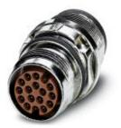
Device connector, front mounting, straight, SPEEDCON locking, M17, Number of positions: 8, Type of contact: Male connector, Crimp connection, Axial O-ring, Central fixing, shielded: yes
