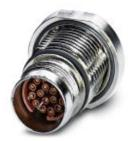
Device connector, rear mounting, straight, SPEEDCON locking, M17, Number of positions: 8, Type of contact: Socket, Crimp connection, Axial O-ring, Central fixing, shielded: yes
