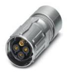
Cable connector, straight, SPEEDCON locking, M17, Number of positions: 3+PE, Type of contact: Socket, Crimp connection, shielded: yes, Cable diameter: 9 mm...11.2 mm
