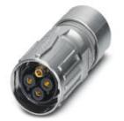
Cable connector, straight, SPEEDCON locking, M17, Number of positions: 5+PE, Type of contact: Socket, Crimp connection, shielded: yes, Cable diameter: 3.5 mm...5.5 mm
