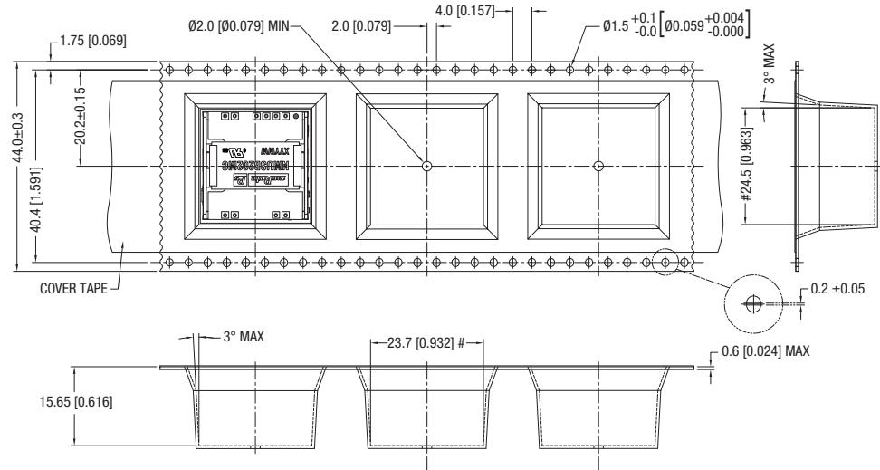
Tape & Reel specifications shall conform with current EIA-481 standard
