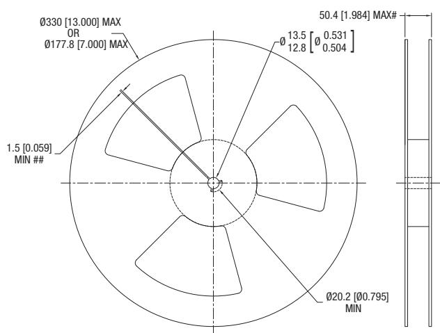
Tape & Reel specifications shall conform with current EIA-481 standard
