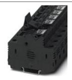
Fuse modular terminal block, Connection method: Screw connection, Cross section: 1.5 mm²- 25 mm², AWG: 16 - 4, Nominal current: 32 A, Nominal voltage: 690 V, Width: 18 mm, Fuse type: Midget / 10.3 x 38, Fuse type: Glass, Mounting type: NS 35/7,5, NS 35/15, Color: black/red
