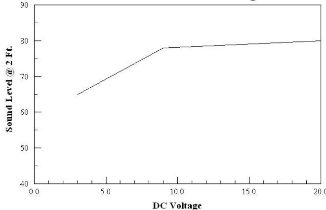
For audible alarm model MSR320R, the sound level will vary from 65 dB at 2 ft. at 3 Vdc up to 80 dB at 2 ft. at 20 Vdc. By varying the voltage from 3 to 20 Vdc, the sound level can be varied by 15 dB. A 10 dB drop in sound level will make the alarm sound half as loud.
