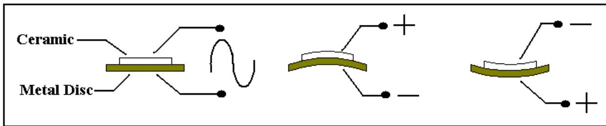
The above picture shows a bare piezoelectric sounder element. By applying a sinusoidal wave-form at an appropriate frequency, the transducer will physically deflect in one direction and then in the opposite direction following the shape of the input wave-form. If this oscillation occurs in the audible frequency range (1 Hz to 20 kHz), then air pressure waves are produced that the human ear interprets as an audible sound.
