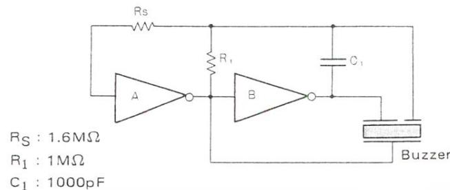
It should be noted that these circuits are only initial suggestions. Values of the resistors may need to be adjusted depending on the particular transducer model used. Square-wave type signals result in more sound level than sine-wave type signals.
