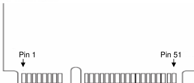
Figure 1-2 Apacer mSATA A1-M pin assignment
