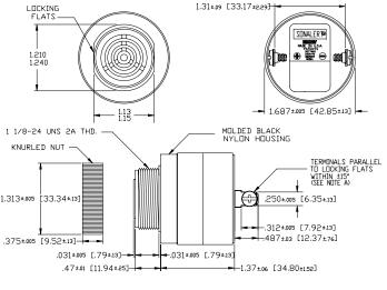
NOTE A: TERMINALS-.032 BRASS TIN PLATED, TAPPED FOR #6-32 SCREW. TWD #6-32 NICKEL PLATED BRASS SCREWS INCLUBED. WILL ACCEPT 1/4\* QUICK CONNECT. NOTE B: MOUNTING- REMOVE BLACK PLASTIC NUT AND INSERT THREADED FRUNT THROUGH 1.25' HOLE PUNCHED IN PANEL, IF DRIENTATION IS NEEDED, NOTE LOCKING FLATS ON DRAWING. SCREW NUT BACK ON. DO NOT OVERTIGHTEN.
