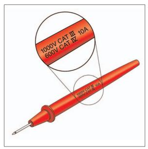
though the DMM is clearly marked with this safety rating, are the test leads equally rated? If the DMM's test leads do not equal or exceed the rating of the tester, then you are putting the tester, and more importantly, yourself at risk.
