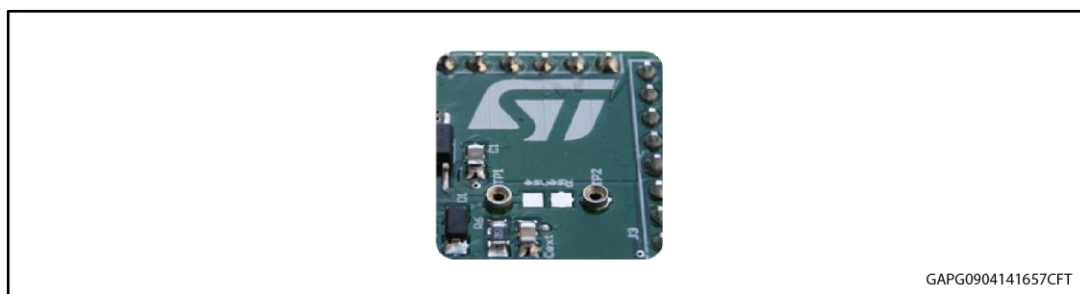
Figure 4: Mounting through-hole sense resistor
