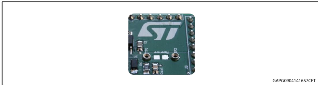
Figure 4: Mounting through-hole sense resistor
