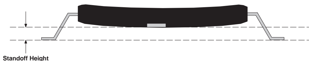
Figure 7-1. Standoff Height Measurement on 144-Pin RFP Package
