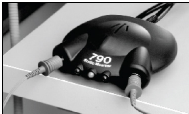
Figure 7. SCS Static Monitor 790 attached to equipment chassis.
