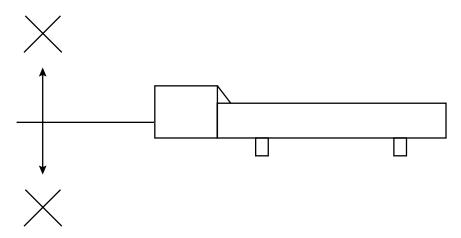
3. When the board warps greatly due to solder flow, the socket may rise up from the board.Please limit as much as possible this board warpage due to solder flow.
