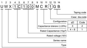
In the case of size φ3 in ( ), parentheses, use WX in the 2nd and 3rd digit and put a 2 in the 12th digit of type numbering system.
