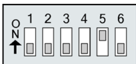
Figure B-18. RS-485 (2-wire) w/ Termination (optional)
