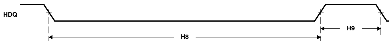
Figure 5-39. HDQ/1-Wire Break (Reset) Timing
