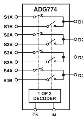
The ADG774 operates from a single 3.3 V/5 V supply and is TTL logic compatible. The control logic for each switch is shown in the Truth Table.
