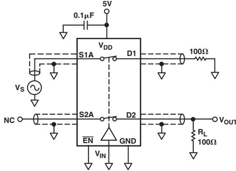
$$\text{CHANNEL-TO-CHANNEL CROSSTALK} = 20 \times \text{LOG} |V_{S2}/V_{OUT1}|$$
