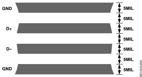
Figure 24. Typical Arrangement of Signal Tracks
