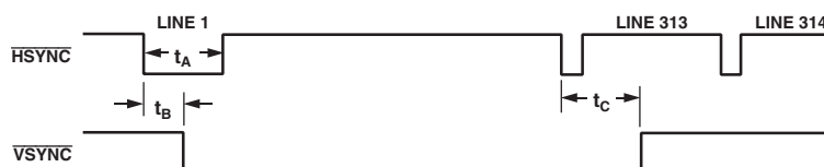
Figure 21. Timing Register 1 in PAL Mode
