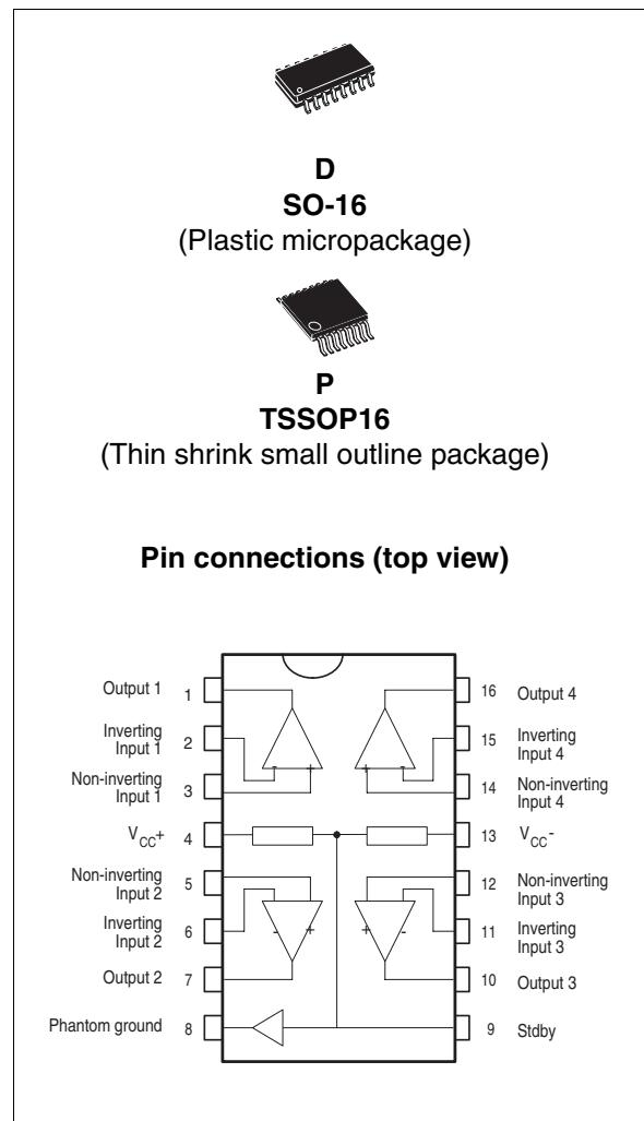
The TS925 exhibits very low noise, low distortion and high output current, making this device an excellent choice for high-quality, low-voltage or battery-operated audio/telecom systems.
