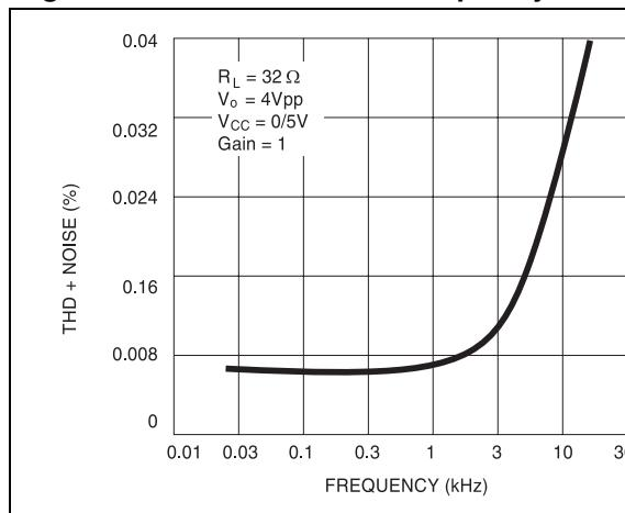
**Figure 12. THD + noise vs. frequency**
