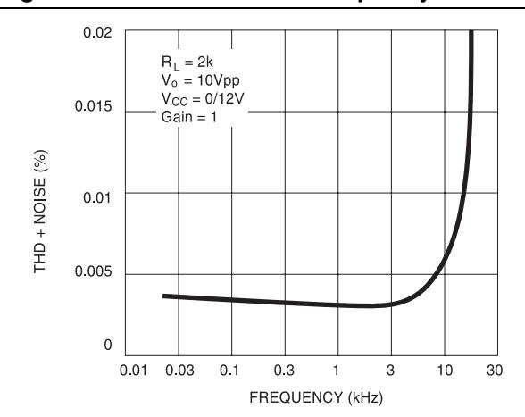
**Figure 11. THD + noise vs. frequency**
