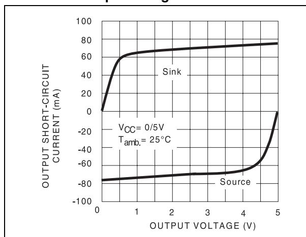
**Figure 6. Output short circuit current vs. output voltage**
