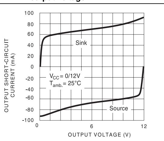
**Figure 5. Output short circuit current vs. output voltage**
