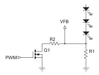
$$\begin{aligned} & \text{MOSFET 'off'} \\ & I_{LED(MIN)} \quad \frac{V_{FB}}{R_{LED}} \\ & \text{MOSFET 'on'} \\ & I_{LED(MAX)} \quad \frac{V_{^{FB}}}{R_{LED}} \quad I_{LED(MIN)} \\ & \text{where V}_{FB} = 100\text{mV} \end{aligned}$$
