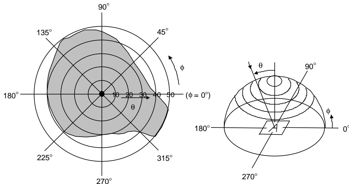
\*Area shows typ.  $CR \geq 2$  (Measuring Spot: 0.9mmφ)
