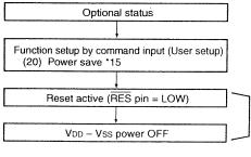
Set the time (tL) from reset active to turning off the VDD - Vss power (VDD - Vss = 1.8 V) longer than the time ( $t_H$ ) when the potential of  $V_5 \sim V_1$ becomes below the threshold voltage (approximately 1 V) of the LCD panel For th, refer to the <Reference Data> of this event. When tн is too long, insert a resistor between V<sub>5</sub> and V<sub>DD</sub> to reduce it.
