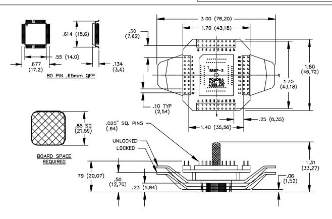
These new test clips provide the user with an easy means to connect instrumentation to the fine pitch QFP chip leads.
