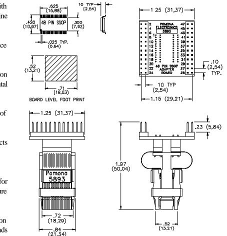
The top interface connects with standard .025" square pins at .100" x .100" spacing. Perfect for use with most logic analyzers.
