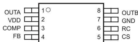
PW PACKAGE (TOP VIEW)
