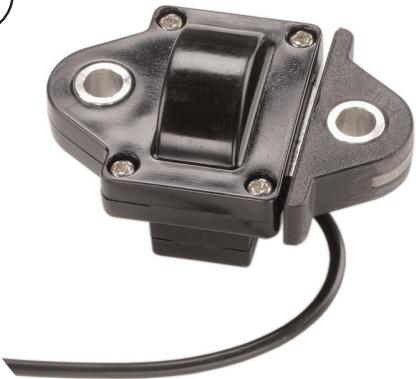
Operating at very low strains, Microfused™ technology provides gage factors greater than 100, an essentially unlimited cycle life expectancy, superior resolution, exceedingly high over-range margins without the need for stops and a ratiometric span of up to 4V. Microfused™ sensors are used in a variety of applications including bathroom scales, paint sprayers and safety-critical automotive brake sensors.
