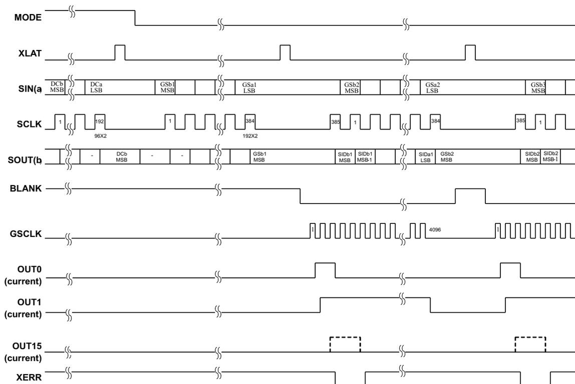
Figure 14. Timing Chart for Two Cascaded TLC5941 Devices
