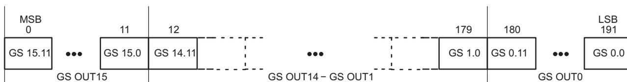
Figure 17. Grayscale Data Packet Format
