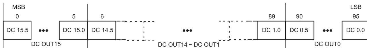
**Figure 15. Dot Correction Data Packet Format**
