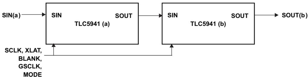
Figure 13. Cascading Two TLC5941 Devices
