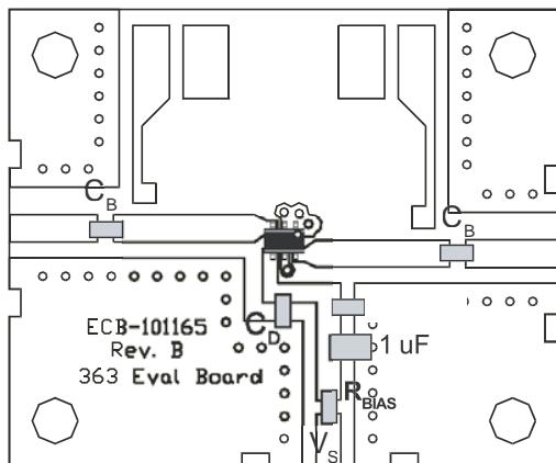
1. Use a large ground pad area near device pins 1, 2, 4, and 5 with many plated through-holes as shown.
