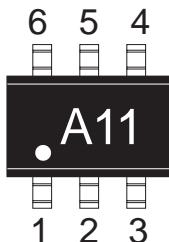
RoHS Compliant part indicated with a "A11Z" on part marking.
