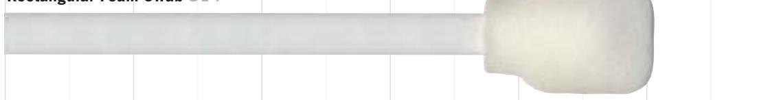
Large foam head bonded to sturdy handle for aggressive cleaning applications. Shred resistant, 100% urethane foam heads with 100 PPI porosity. Bonded securely to a 5" polypropylene shaft.
