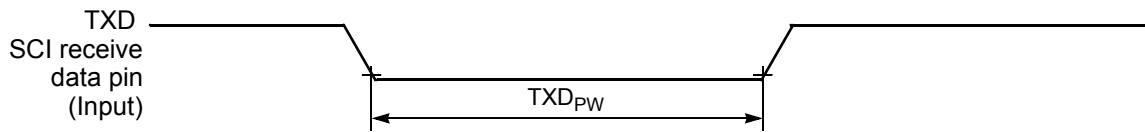
Figure 10-17 TXD Pulse Width
