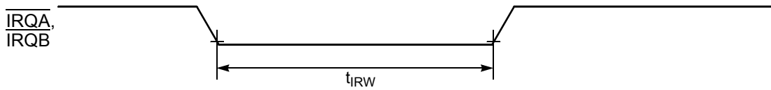
Figure 10-6 External Interrupt Timing (Negative Edge-Sensitive)
